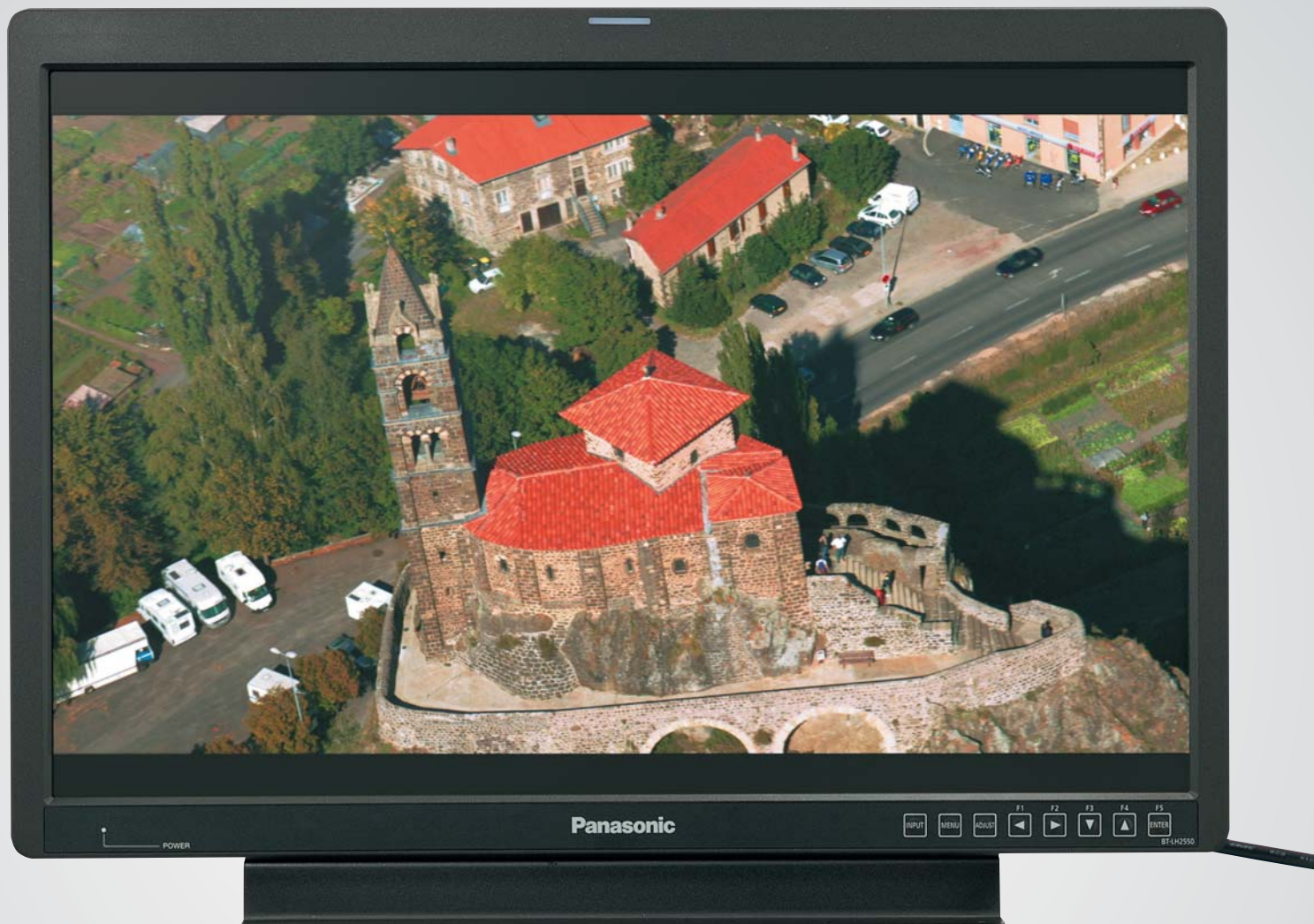
A sample image recorded by an AVC-Intra 100 codec. It is a still image captured from 1920 x 1080-pixel video recorded using 10 bit/4:2:2 sampling.
